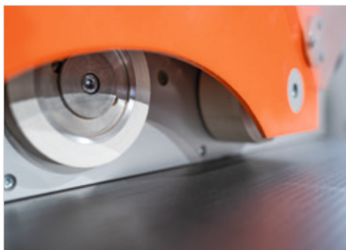
Circular saw feeder 76: Infeed roller in detail
